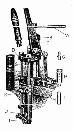
The new No. 45 Lubricator and Sizer employs the same type of sizing dies used in the No. 1 Lubricator and Sizer, enabling the owners of the older sets of dies to use them in the No. 45 Tool.
